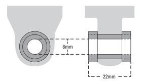
Once you found the right length and stroke, please make sure the mounting size of your frame fits to the selected SRSUNTOUR rear shock. The image on the left shows our factory standard setup. Different widths and diameters are available on demand.
