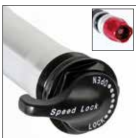
LO R: Rebound adjust + speed lock out
