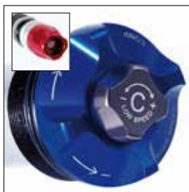
RC2: High & Low speed Compression adjust
